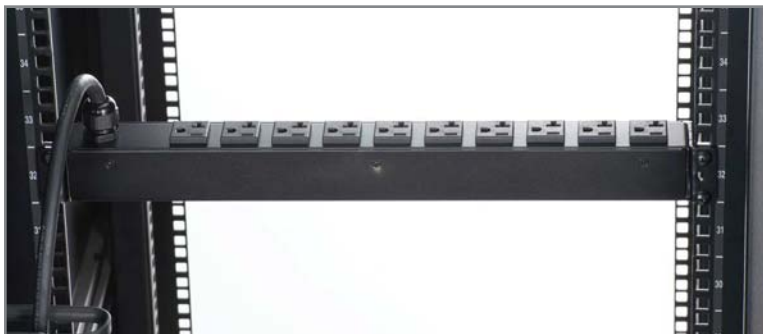
120V, 20A Basic PDU with NEMA 5-20 receptacles shown at the back of the rack with the receptacles facing up. This orientation is useful for preventing plugs from being pulled out.
